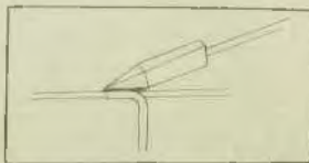
How to apply the soldering iron. Note the flux resting on the busbar.
