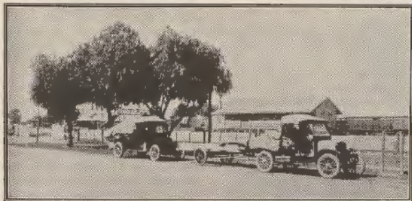
Outfit at Nyngan. "The Flea" with improvised trailer attached. The trailer was made from the wireless masts.
