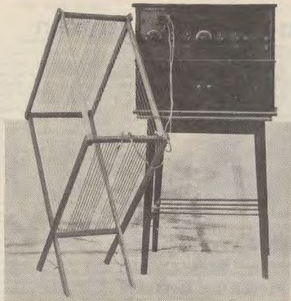
The Completed Receiver with Loop.
