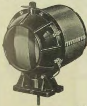
VARIOCOUPLER. R125 The finest that can be produced. Moulded brown bakelite, split bronze bearings winding tapped at 15 points for very close tuning. Obtainable in two sizes.
