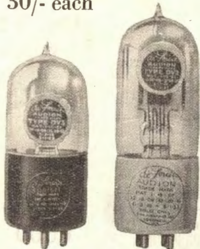
D.V.3 D.V.2 Filament, 3-v. Filament, 5-v. .06 amp. .25 amp. Both types fit standard American Socket.
