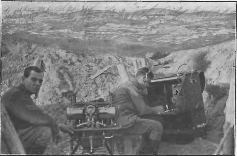
A MESSAGE BEING RECEIVED ON A PORTABLE WIRELESS STATION IN A TRENCH.
