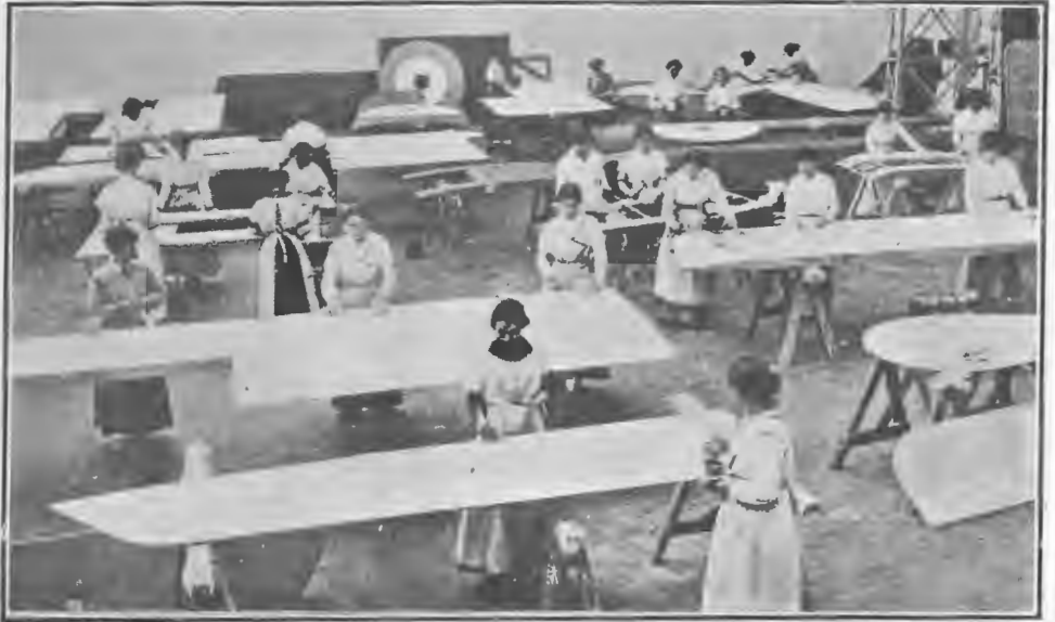
THE MANUFACTURE OF SEAPLANES—A VIEW OF THE DOPE ROOM.
