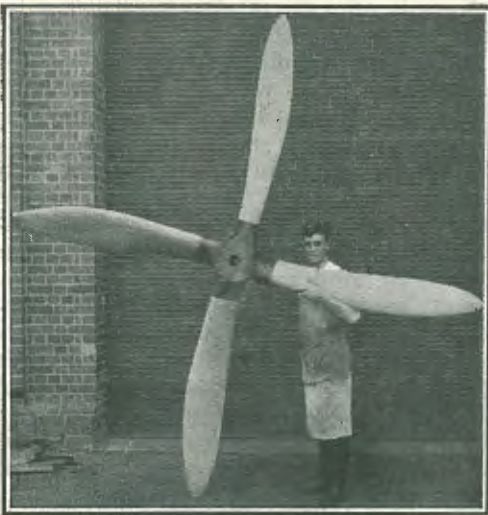
Propeller of Queensland maple, made out of stock in Ipswich Shops.
