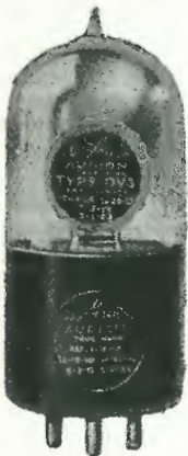
D.V. 3 Filament, 3 Volts, .06 Amp.
