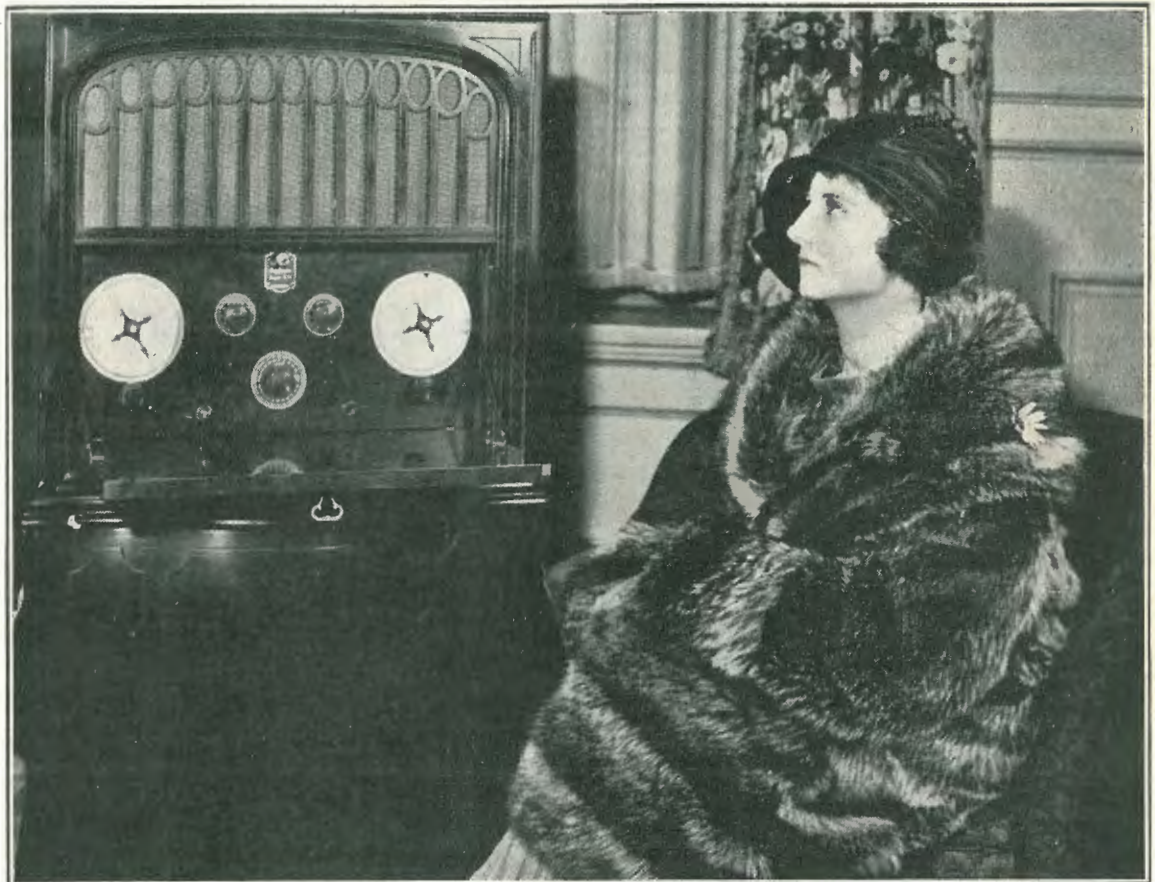
An example of an effective radio installation at broadcasting station WJY, New York City. The receiving set is a Radiola Super-VIII.
