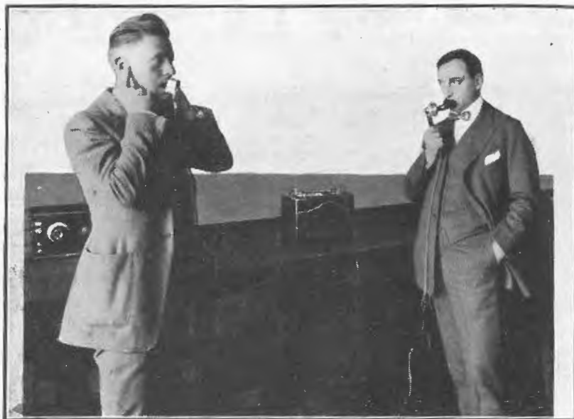
How the invention is used to talk to a person who is hard of hearing. To hear with the "Osophone" the normal person must close his ears tightly when the sound transmission is completely through the teeth. In this experiment an ordinary telephone transmitter connected with a 6-volt battery was used.
