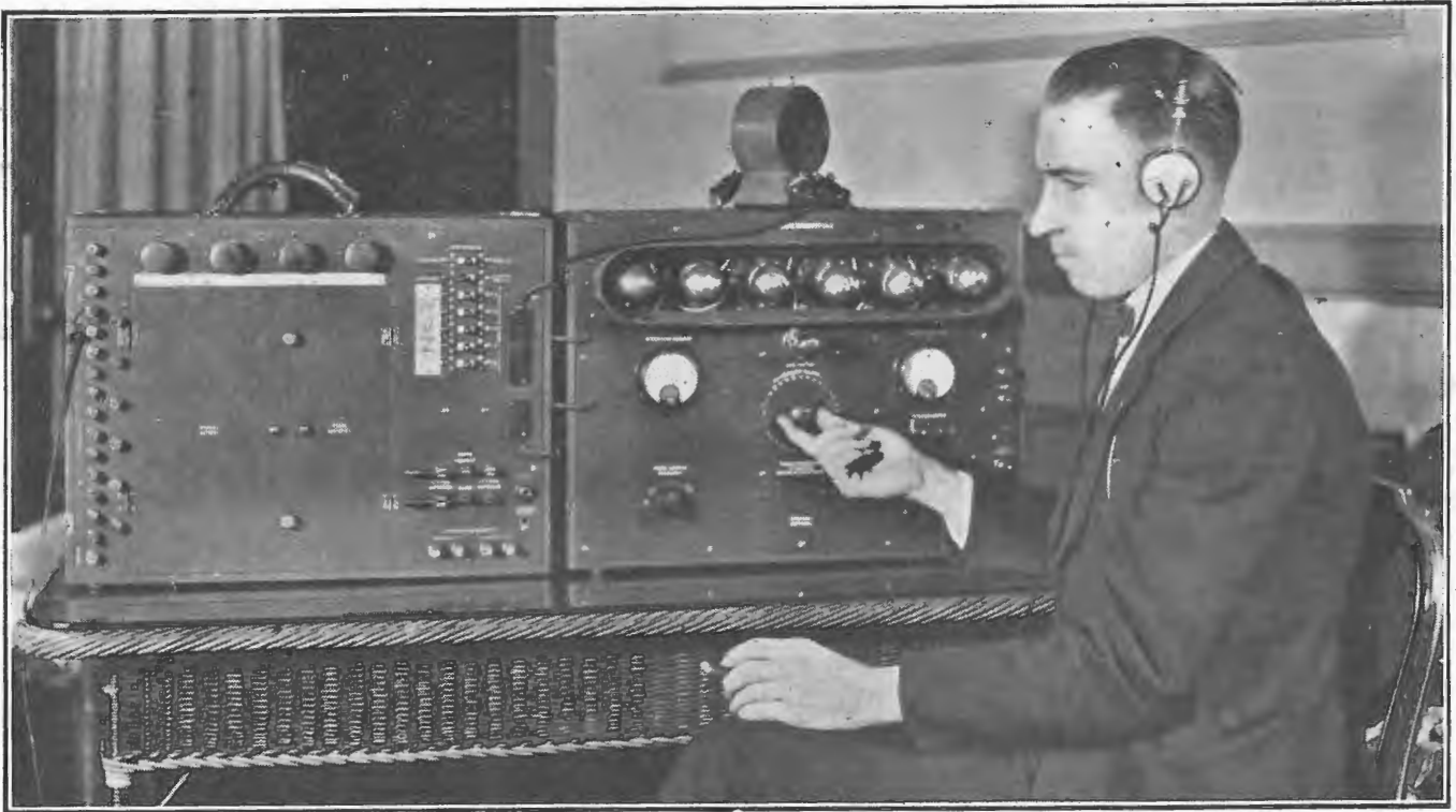
Operator adjusting "line-amplifier" at Station WJY, thus regulating the quality and strength of the broadcasted music and speech.
