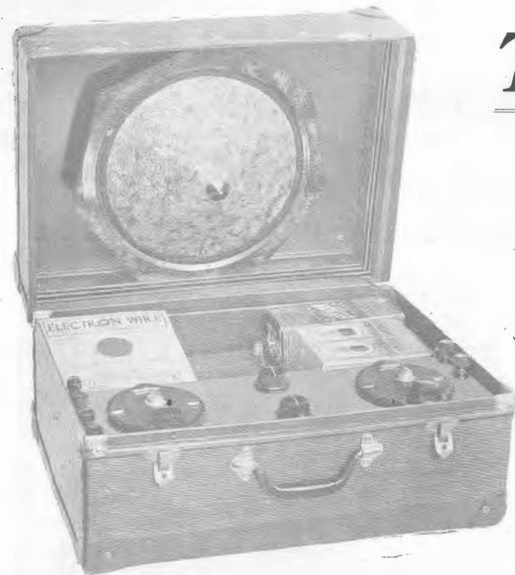
FIG. 1.—The Holiday Portable, as it appears in use. The loop aerial is wound inside the lid, which also holds the cone speaker.
