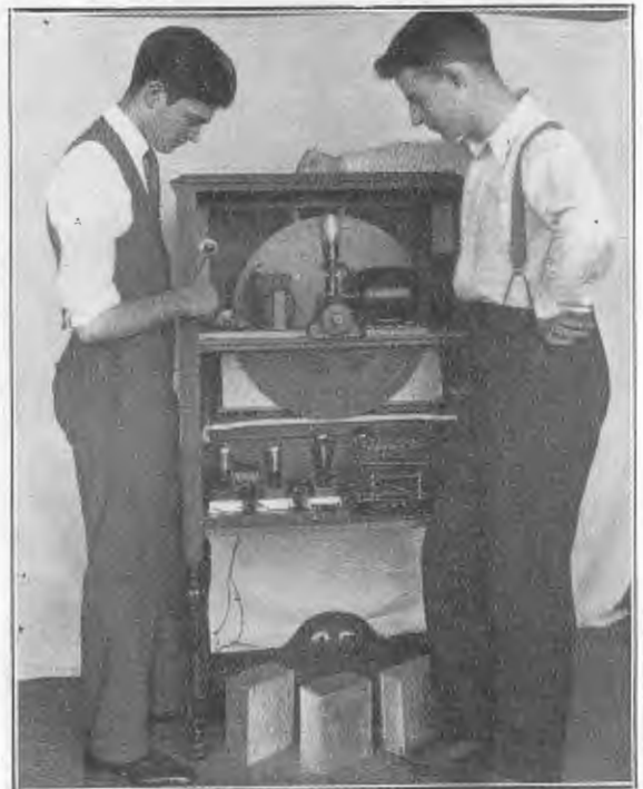
What the inside of the complete Radio Broadcast and Television Receiver looks like. The receiver proper occupies the lower section of the cabinet, the television apparatus the upper.
