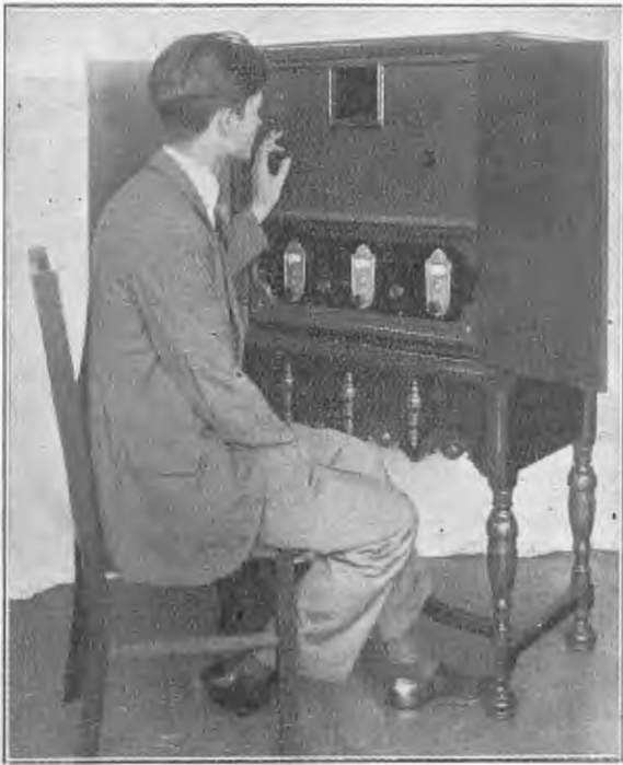
John Geloso, who designed the machine, is here shown adjusting the complete television receiver, and is observing a picture through the square opening in the cabinet.
