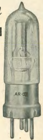
TYPE "A. R. 06." Filament Voltage, 2.5. Plate Voltage, 20-50. Filament Current, .06 amperes. Price, 13/6 each.
