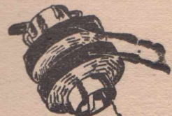
Line filter coil.
