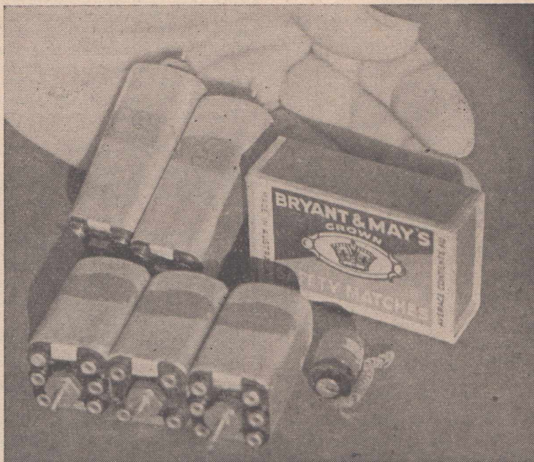
A photo of the Q-Plus coil kit for car radio, with a match-box for comparison of size.
