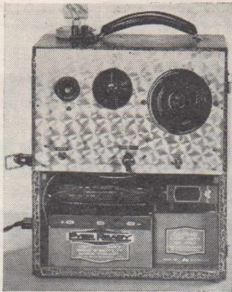
"The Companionette Three," a three-valve a.c. receiver with the gain and selectivity of a "four." (March and April, 1937).
