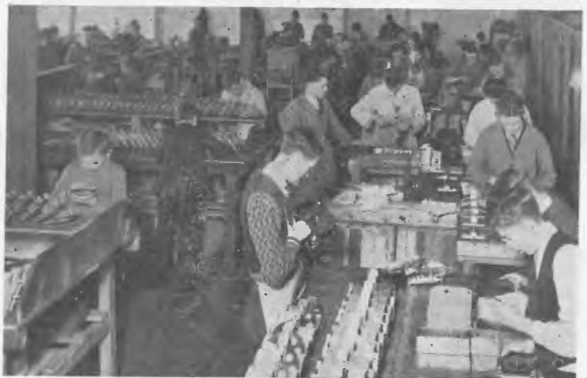
In this section (below) of the production department, dials are assembled under the mass production system, with inspectors checking every stage of the assembly.
