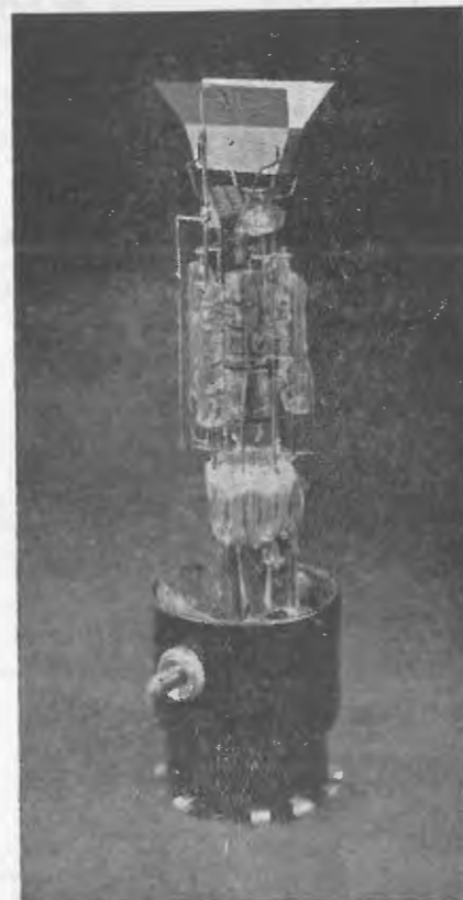
An "exploded" view of the DG7-1.
