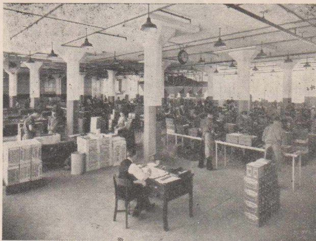
Another view of the cell assembly department. The huge hoppers in the background contain the cardboard tubes used as insulating containers for the cells.
