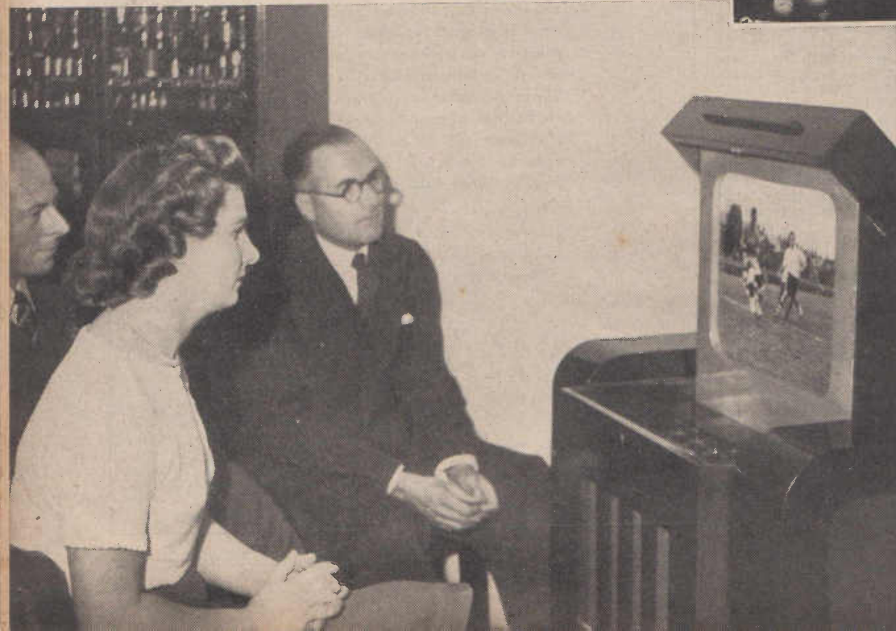
● The new process of projecting television images on to a large flat-surfaced screen. The system has been perfected by the Mullard Wireless Service Company, Shaftesbury Avenue, London, England. The ample size and clarity of the picture is evident from this striking photograph.
