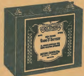
Columbia 45 Volt Vertical "B" Battery No. 4772. Designed for all sets having not more than five tubes using 90 volts. Occupies less than half the table space of the horizontal 45 volt battery, yet contains the same large powerful cells. Three Fahnestock spring clips—negative, plus 22½, and plus 45 volts. .... 25/- each.
