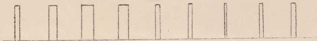
(c) Pulse-Width Modulation. Pulses constant repetition - Frequency variable width.
