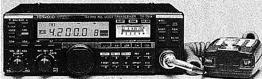
Start with a rig like this and you won't need to upgrade when you upgrade your licence. This is Kenwood's TR-751A all-mode rig featuring both 2 m and 70 cm operation.
