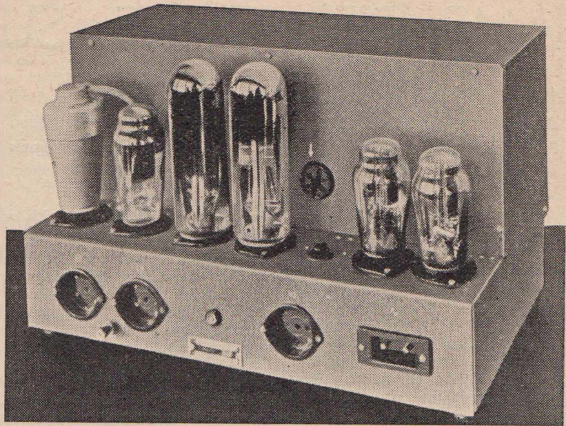
In spite of the fact that this inverse feedback amplifier is capable of an undistorted output of 50 watts, it is extremely compact.
