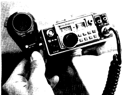
Transceiver and microphone. Microphone has a scanning switch.
