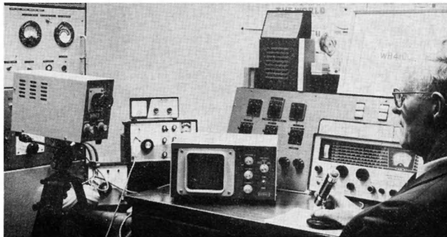
Stan VK3TE at the controls of his "Robot" camera and monitor. This camera has facilities for fast scan output, a good feature for rapid focus and set-up.
