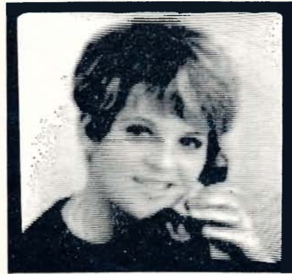
Fig. 4.—Picture taken from a commercial monitor of U.S. origin and readers should observe the pin-cushion effect that occurs on most 25-inch tubes today.
