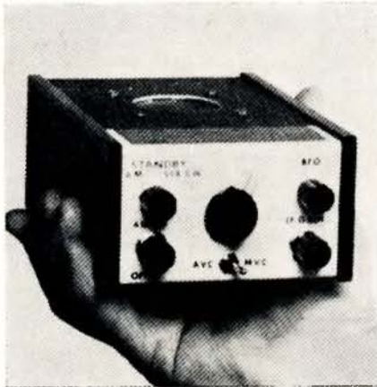
K4DHC's miniature 75 metre Receiver utilising the LM373 in the i.f. system.
