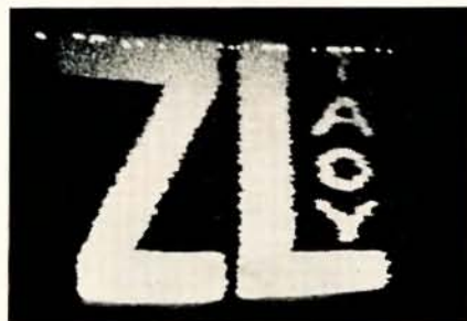
Call of ZL1A0Y received by John VK3LM (white letters on black background) on FT200. Strength S8, noise-free picture. Sync. pulling seen on picture. Taken from monitor of Mac VK3YEO.
