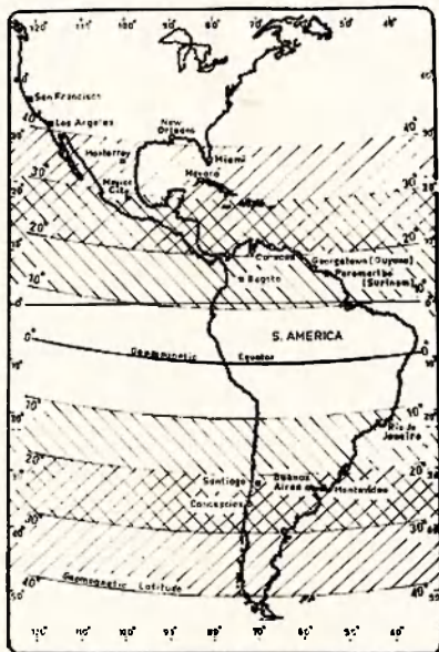
Fig. 3.—The American sector of the world showing terminal zones for Class I. TEP (20 deg. to 40 deg. geomagnetic latitude) and Class II. TEP (10 deg. to 30 deg. geomagnetic latitude).
