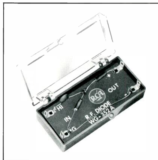
RCA's new diode assemblies (WG-352A shown above) extend instrument capability by rectifying and filtering a high-frequency signal so it can be measured by a conventional VOM or oscilloscope.
