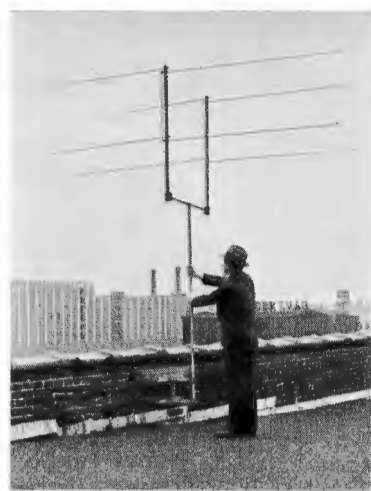
The reflector on this RCA Double Di-Pole Television Antenna, Stock Nos. 9871 and 9872 gives improved reception from one direction and rejects signals from the other
