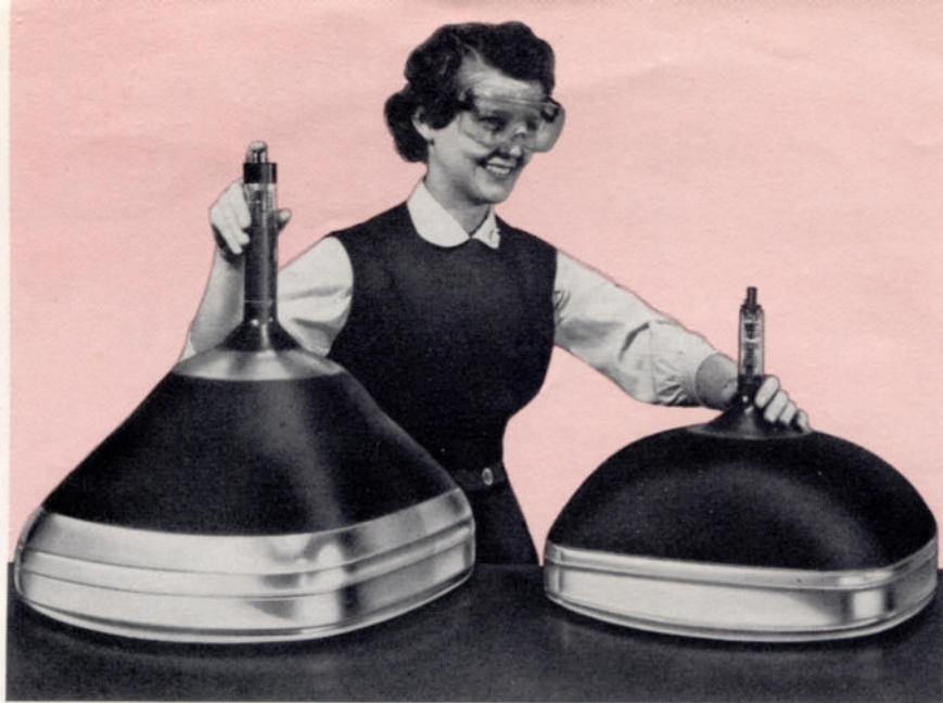
More compact TV sets are in the offing with such "110-degree" picture tubes as the RCA-21CEP4 (right) which has an overall length that is approximately 5½ inches shorter than the tube (left) having the same size faceplate and 90-degree deflection.
