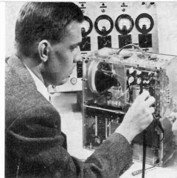
Gerald B. Herzog, of the RCA research staff, makes laboratory tests on an experimental battery-operated television receiver which uses developmental and experimental transistors and no tubes except the 5-inch picture tube.
