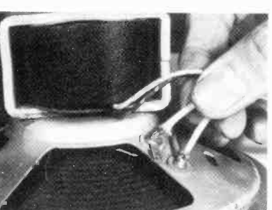
44. In cases where the intermittent-contact trouble affects the sound, don't forget to check the speaker. Check the voice coil, field coil, output transformer, cable, plug, and socket.
