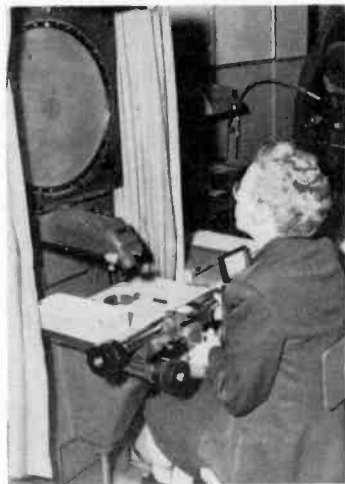
Samples of the basic structural components of the tube are carefully tested for strength and uniformity before the lot is sent to the plant for use in tube manufacturing. The test on the right measures mica wafer dimensions by means of a 30-power projection microscope. Detailed specifications for each type wafer must be met to within close tolerances. The machine on the left is a ductility tester. It measures the strength of the pins used in miniature tubes, assuring only the finest materials for RCA tubes.
