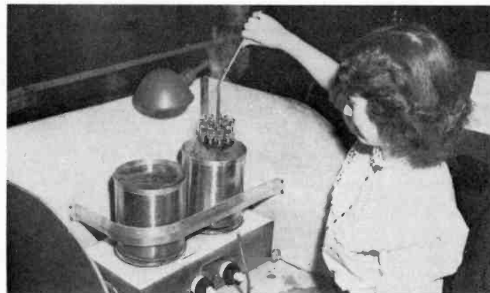
This is known as the "B Test". Completed tubes are forced over cones and dipped into boiling water, then into cold water. Breakage is analyzed and excessive strains are corrected in the base manufacturing stage.
