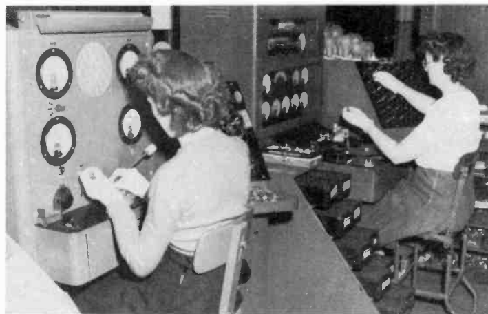
Two of the many test units devoted to thoroughly checking miniature tubes to make sure of uniform quality and maximum service life in the field. The unit at the left is the microphonics test set, where the slightest trace of microphonics is audible to the operator. The right unit tests the miniatures for shorts and emission. Every tube either passes both tests or is destroyed. Samples of each batch are tested again before final shipments.
