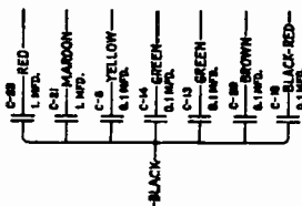
INTERNAL CONNECTIONS OF BY-PASS CAPACITOR
