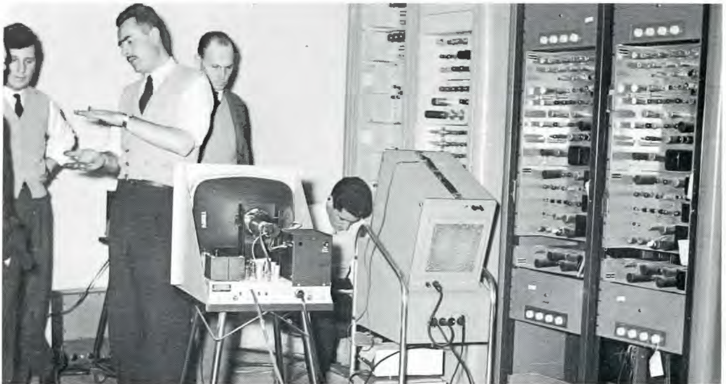
Argentine technicians work on studio control rack equipment at new Channel Nine Station in Buenos Aires.
