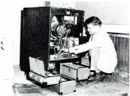
Virgil Talbot makes a rear chassis adjustment to a color television set
