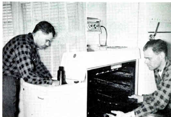
Appliance serviceman Ken Spears removes the agitator from a washer (l.) and checks a range's oven
