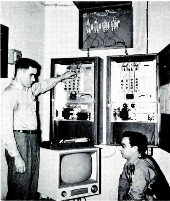
Bob Sherrill (standing) adjusts gain of amplifier while Vern Tantillo checks on picture quality
