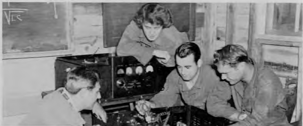
FRANK E. COLONNA, also 645th AC&W Squadron, Roslyn, familiarizes two Sergeants and a PFC with layout of BC-610 transmitter components. RCA supervised on-the-job training greatly helps students understand equipment.
