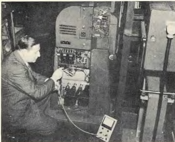
Ray Norton, Service Engineer of Philadelphia district, checks an RCA TV Film Projector at WFIL-TV, Philadelphia.
