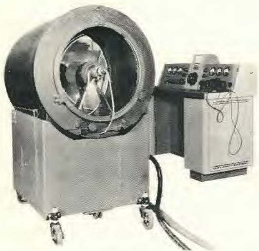
Fig. 1—Television Projection equipment employing 30-inch spherical mirror and 22½-inch aspherical correcting lens.
