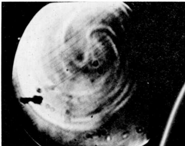
Fig. 8—Microscopic inhomogeneity in 1 inch diameter silicon crystal.
