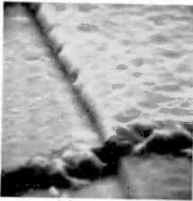
Fig. 10—Scanning electron micrograph of Al film cross section over a sputter-etched edge (argon pressure = 2.5 mtorr., bias = 0, B = 0 ).
