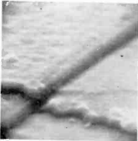
Fig. 10—Scanning electron micrograph of Al film cross section over a sputter-etched edge (argon pressure = 2.5 mtorr., bias = 0, B = 0 ).
