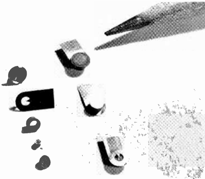
Fig. 2—Varactor diode parts and assembly.
