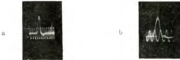
Fig. 37—Detected pulsed carrier signal generator output. (a) Sawtooth time base with 55-megacycle markers. (b) Pulse time base with 55-megacycle markers.
