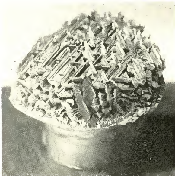
Fig. 4—Another view of the recrystallized germanium showing the hollow (111) facets.
