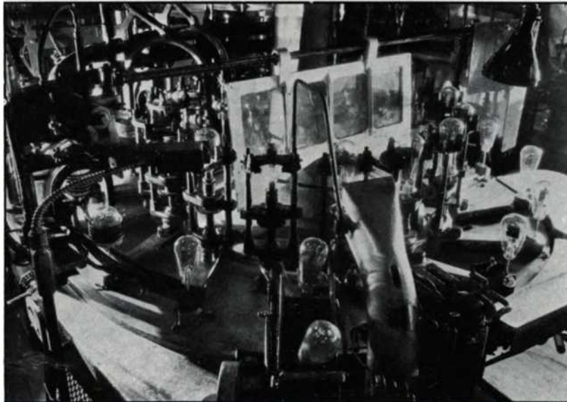
Fig. 13. The Sealex Machine seals and exhausts the tube—hence the name Sealex
