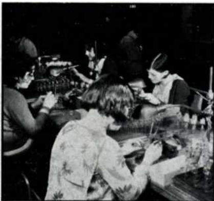
Fig. 10. Here the parts are skillfully assembled on the stems
