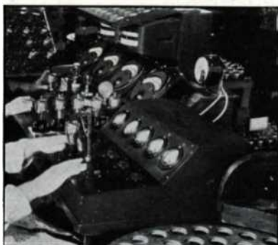
Fig. 15. Final factory check on tubes before packing. Any tube which does not qualify is rejected—there are no "seconds"!
