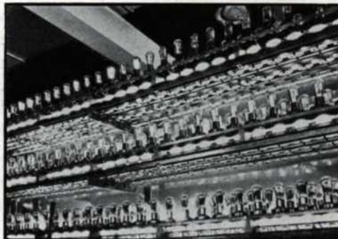
Fig. 16. Seasoning racks where tubes are "tempered" for stabilization of characteristics
