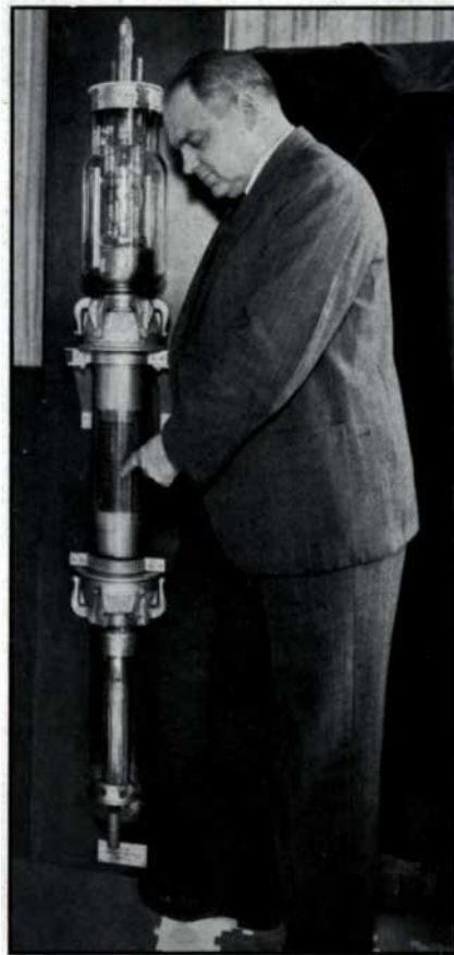
O. H. Caldwell standing beside world's largest vacuum tube, the Westinghouse AW220, a 200,000 watt transmitting tube whose grid and plate are water-cooled. Five tons of water are required for this purpose hourly
