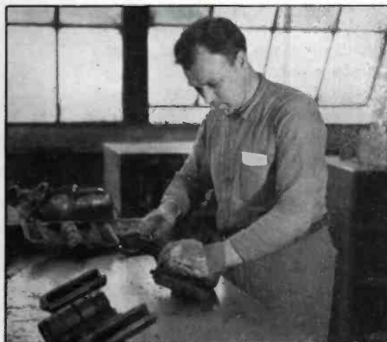
The bulb molds have to be scraped, tested, and recoated every eight hours
