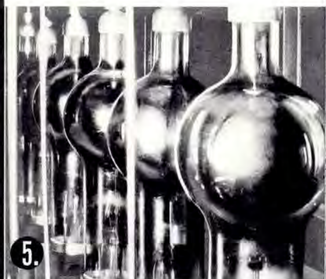
A boost along the way —Now the music of the Magic Key artists has reached a station of the NBC Blue Network. It has traveled by wire from the giant switchboard. Before being broadcast it must be boosted up to greater strength. Above you see a battery of RCA power tubes which do this job. These tubes are costly. WJZ, famous NBC station, makes use of more than 60 tubes when it is on the air.
