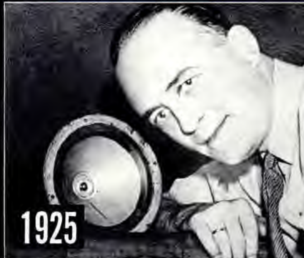
THE DYNAMIC SPEAKER was big forward step toward greater range of notes and volume without squawking. Picture above shows early example of this famed invention.
