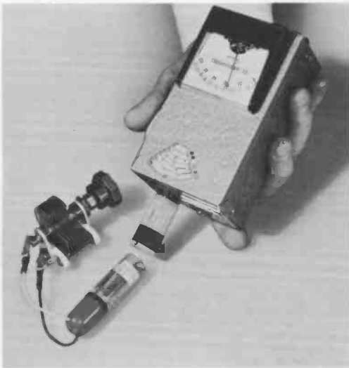
Figure 1: Use of author's grid-dip meter to measure value of an unknown capacitor. The standard inductance consists of 15¼ turns of B&W Miniductor #3003 (½-inch diameter, 16 TPI) enclosed in an Amphenol coil form type 24-5H. Note use of adapter with clip leads for connection to unknown capacitor.
