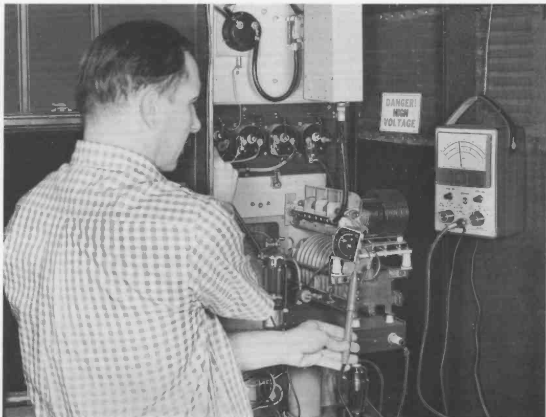
When connected to a wavemeter circuit, the VoltOhmyst makes an excellent rf-tuning indicator. Here, W2IYG uses the WV-77C and WG-301A Crystal-Diode Probe during neutralizing of final amplifier.
