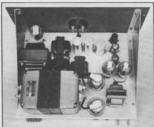
Fig. 2. Top view of the modulator; note that the well-planned layout of the modulator components permits the inclusion of a husky power supply on the same chassis.
