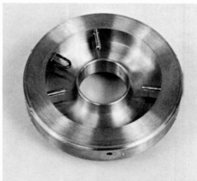
Fig. 4—A half section of the RCA 8568 klystron fourth cavity showing cavity loops and mode suppressors used to stabilize the tube.
