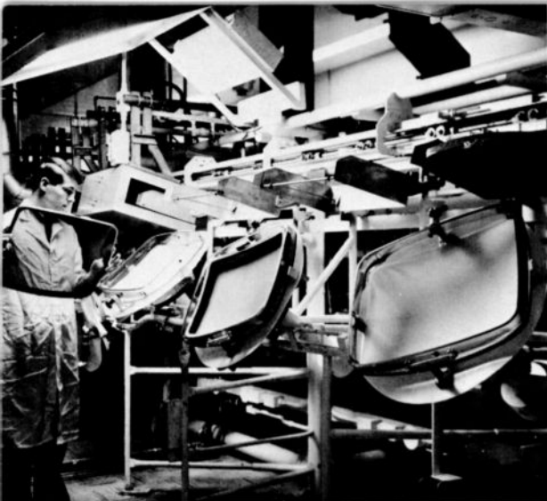
Inserting the shadow mask after phosphor application.
