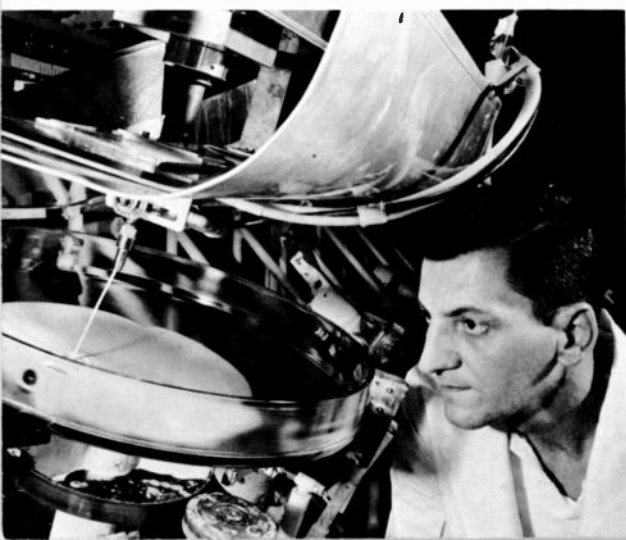
Phosphor slurry being dispensed.
