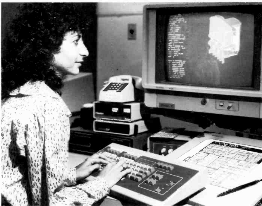
Fig. 4. Control Data CAD station at RCA Laboratories. Here, solids modeling is being used to examine the assembly of a picture tube gun.
